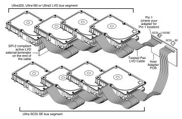
Figure 3. Cable connections and external termination
